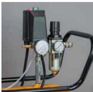
Control unit equipped with a cup filter for cleaning the compressed air outlet.
