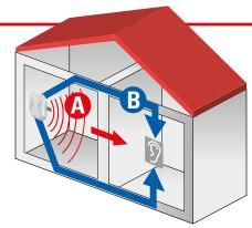
construction elements, such as the floor and the ceiling. For example, a washing machine during the spin cycle. Materials propagate sound differently: dense, solid, and heavy materials (glass, concrete, or stone) vibrate less than light, thin materials. They produce high noise levels while porous materials (foam or perforated products such as wood panels or plaster) absorb noise better.
