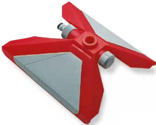
Ballasted sled, inlet with M coupling or thread. 3/4" M Thread. outlet F 1/2" Allows in-series connection
