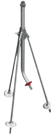
Galvanised iron tripod thread. 1" M and thread.adaptor 3/4" M Inlet with Ø 25 mm barbed connector Height-adjustable from 60 to 80 cm
