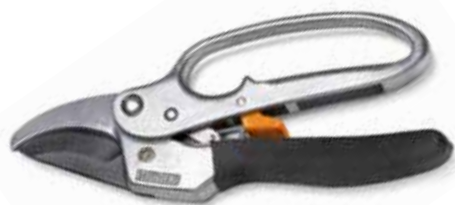
Ratchet shears with curved hardened steel blade, non-stick coating, counter-blade with branch lock grooves, aluminium handles with anti-slide thermoplastic covering and finger protection arc
