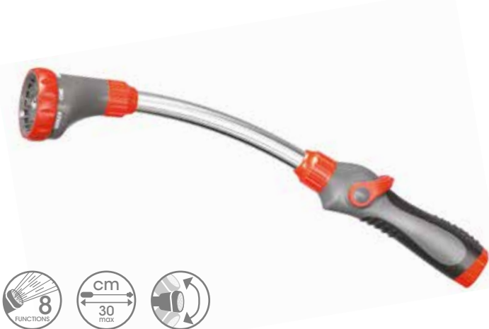
Aluminium shower spray nozzle, 8 functions, multi-jet, 30 cm long. Anti-slide ergonomic handle with adjustment and locking slider
