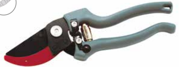
Anvil pruning shears, 21 cm, Teflon-coated curved interchangeable blade, ergonomic handle with anti-slide coating blade in hardened carbon steel HRC 54:56
