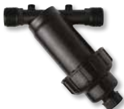
1" M - 1" M filter Filtering cartridge in 155 stainless steel Mesh (100 Micron) Maximum flow rate 80 l/min Maximum operating pressure 10 bar Body and plug in Nylon Drainage plug Ø 1/2" F for quick cleaning
