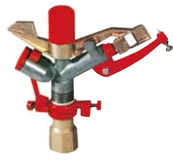
Adjustable sector brass sprinkler Standard Ø 6 mm nozzle
